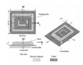
Fig 5. Geometry of a U-slot rectangular patch antenna printed on a microwave substrade.
