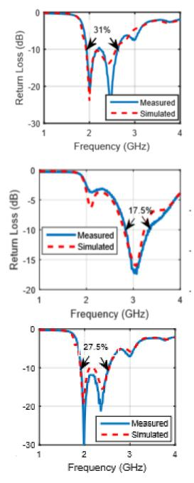
Fig. 2. Measured and simulated return loss on (r = 4.4, h = 11.811 mm) for (a) DIResF (b) DI (mod) (c) ResF (mod)
