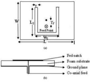
Fig 10 (a) Top view of the proposed antenna, (b) Slide view of the proposed antenna
