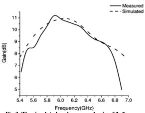
Fig.3. The simulated and measured gain of 2×2 array.
