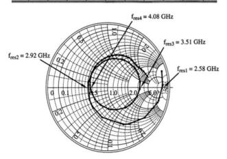
Fig.6 Stimulated input Impedance of the initial U-slot microstrip patch used in the parametric studies. The four resonant frequencies of the structure are indicated
