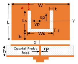
Fig.1. U-Slot loaded microstrip patch
