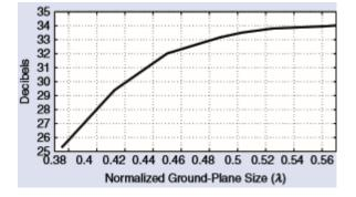
Fig. 9 The difference between the copolar and crosspolar levels versus the normalized groung-plan size
