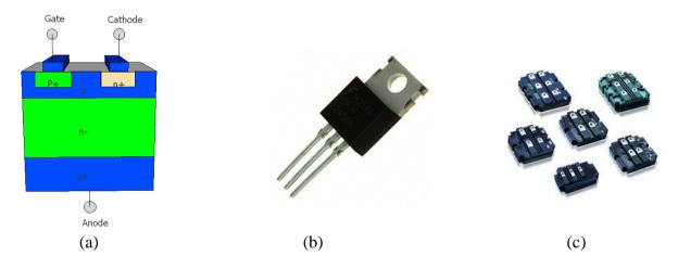
*Figure 1.* (a) Gate turn off thyristor representation with PN layers, turn on accomplished by positive current between gate and cathode (b) Power MOSFET (c) Insulated gate bipolar transistors
