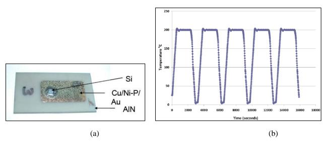
*Figure 12.* (a) Chip module assembly arrangement. (b) Thermal heat cycling method. *Minimum temperature of*  $5^{\circ}$ C *and maximum temperature of*  $200^{\circ}$ C *applied.* [16]
