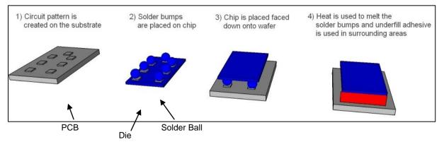
Figure 4. Flip Chip Process
