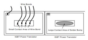
Figure 7. Wire-bonding compared with solder bumping/posts
