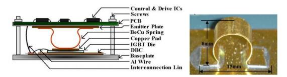
Figure 9. Pressure contact assembly [11]
