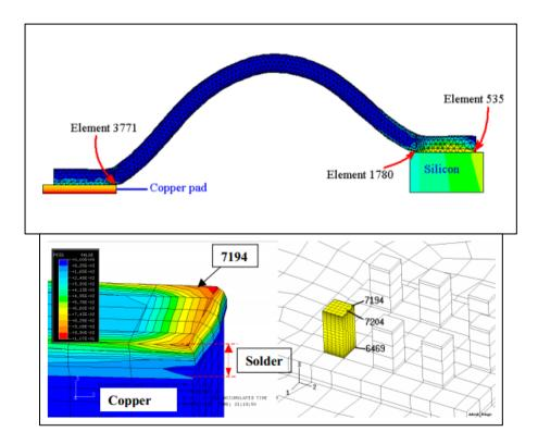
Figure 10. Finite element software analysis of wire bonding and MPIPPS structures [5]
