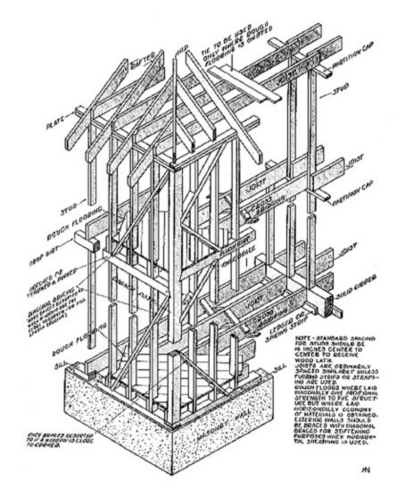
Figure 4. Braced Framing pre-1900.
