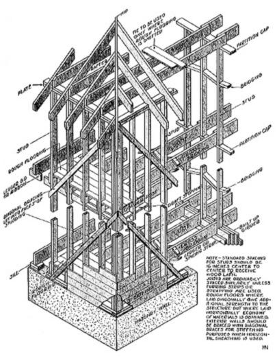
Figure 5. Balloon Framing Technique in Early 1900s.
