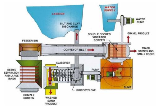
Figure 10: Dutch Pilot Plant for separating litter and trash from dredged material (from Spaine et al., 2001)
