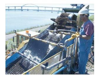
Figure 8: Example of vibrating screen (from Spaine et al., 2001)
