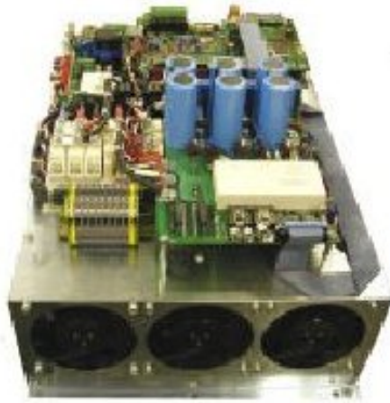
Fig. 3.10. Youtility's 25 KVA power converter.
