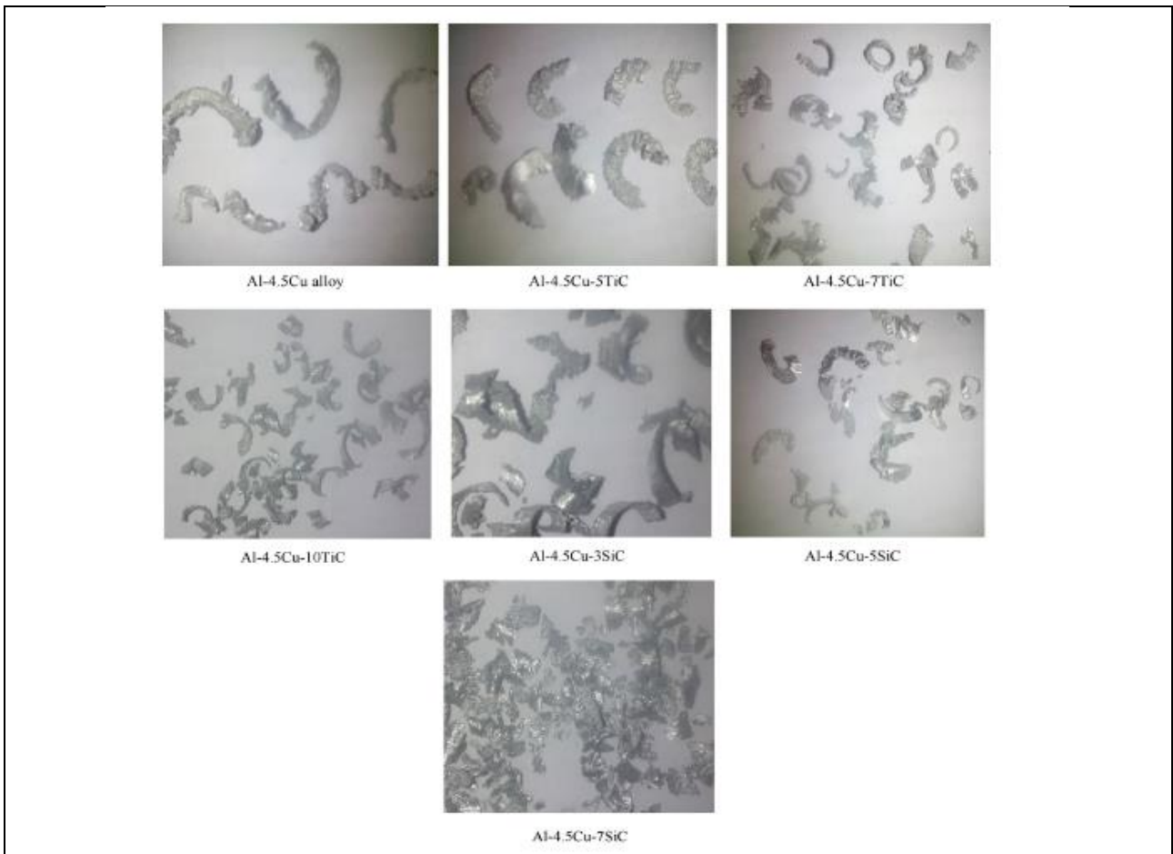
Fig. 7. Chips formed during machining process of Al-4.5Cu alloy, Al-4.5%Cu-TiC and Al-4.5%Cu-SiC respectively
