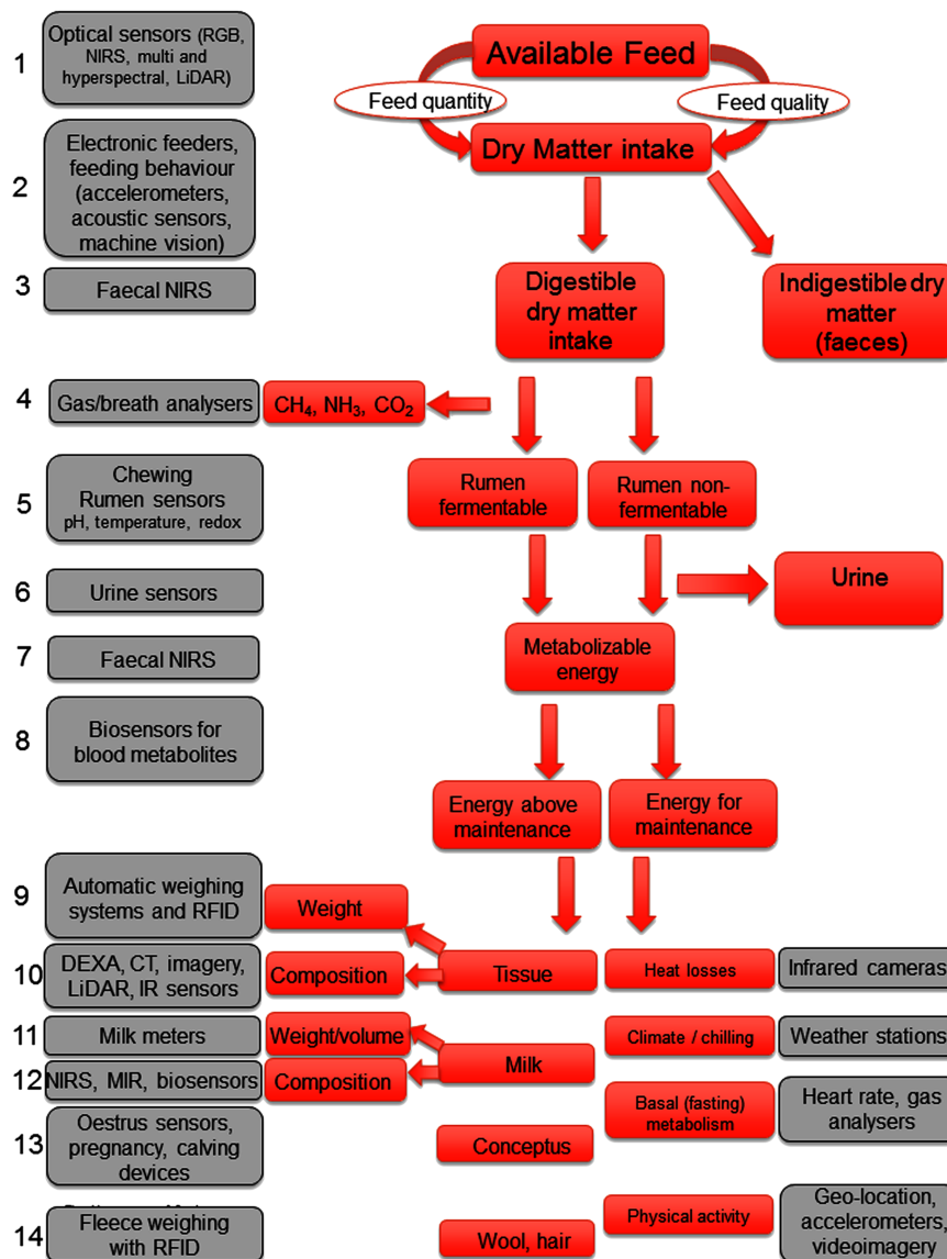
Figure 1 A simplified hypothetical flow of nutrients through an animal (red boxes) with potential technologies to measure key nutritional processes (gray boxes). RGB = red, green and blue; LiDAR = light detection and ranging; DEXA = dual energy X-ray absorptiometry; RFID = radio frequency identification; CT = computer tomography; MIR = mid IR.
