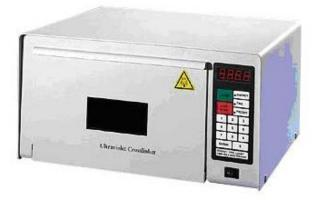
**UV Crosslinker**- Used to attach nucleic acids to a surface or membrane following blotting procedures. Crosslinkers are equipped with door safety interlocks, which similar to a household microwave, prevent operation of the machine when the door is open. If the interlock system is not functioning correctly, refrain from using the device and contact the manufacturer.
