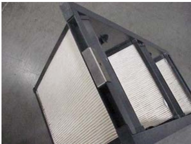
Filter Plug Installed
