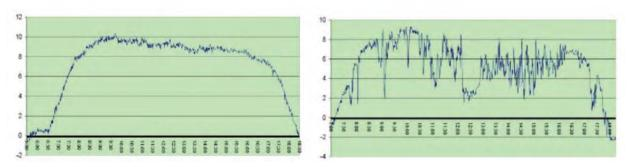
Figure 29 - Nevada Solar Photovoltaic (PV) Plant Output on a Sunny Day (Left) and a Partly Cloudy Day (Right) in 2008. Source: MIT study "The Future of the Electric Grid"
