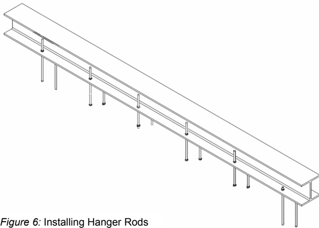
Figure 6: Installing Hanger Rods
