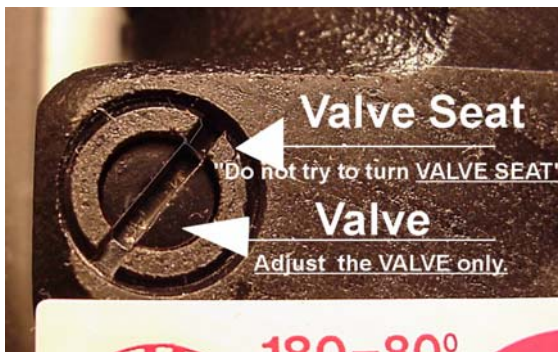
Fig. 52 use small blade screwdriver only
