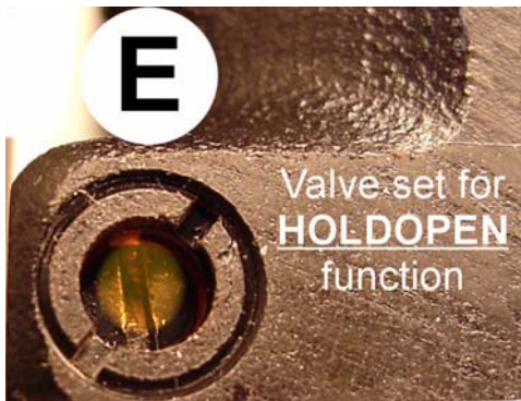
Fig. 53 Position of valve for hold open operation
