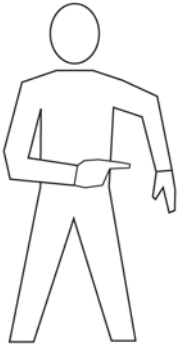
Arms extended with forearm perpendicular to ground. Palms facing body. Gesture indicates right side. HOT BRAKES - RIGHT
