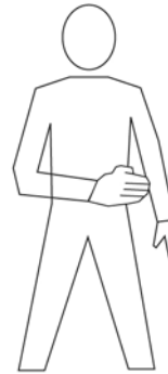
Raise arm, with fist clenched, horizontally in front of body, and then extend finger RELEASE BRAKE
