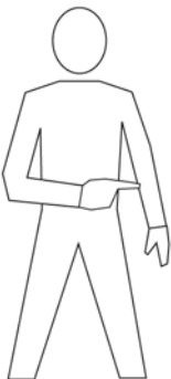
Right or left arm down, other arm moved across the body and extended to indicate direction of next marshaller. PROCEED TO NEXT MARSHALLER
