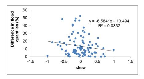
Figure 2.34 Plot of skew of log<sub>e</sub>(Q) vs. differences in flood quantile estimates between CV of 0% and CV of 20% (96 catchments from NSW) (for 2% AEP flood)
