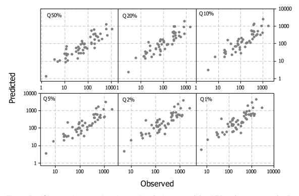
Figure B.2 Observed vs. predicted quantiles (in log space) for AEPs of 50% to 1% for Region 2 (Tasmania) (flood discharges are in m³/s)
