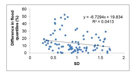
Figure 2.33 Plot of SD of log<sub>e</sub>(Q) vs. differences in flood quantile estimates between CV of 0% and CV of 20% (96 catchments from NSW) (for 2% AEP flood)
