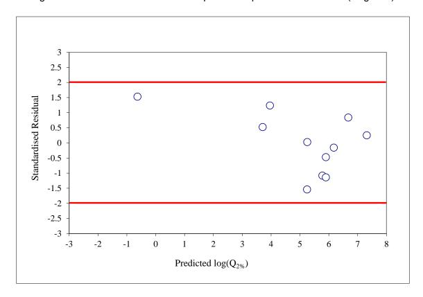
Figure C.4 Standardised residuals vs. predicted quantiles for 2% AEP (Region 6)
