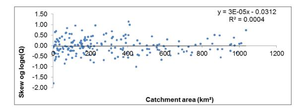
Figure 2.39 Relationship between skew of log<sub>e</sub>(Q) and catchment area for NSW 176 catchments
