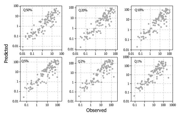
Figure B.8 Observed vs. predicted quantiles (in log space) for AEPs of 50% to 1% for Region 5 (SW Western Australia) (flood discharges are in m³/s)
