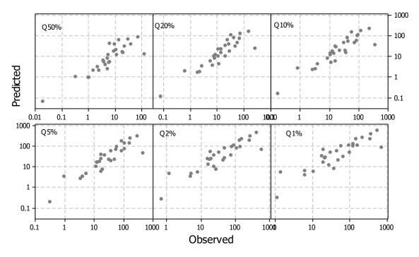
Figure B.4 Observed vs. predicted quantiles (in log space) for AEPs of 50% to 1% for Region 3 (South Australia) (flood discharges are in m³/s)
