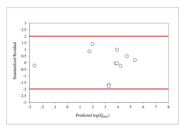
Figure C.1 Standardised residuals vs. predicted quantiles for 50% AEP (Region 6)
