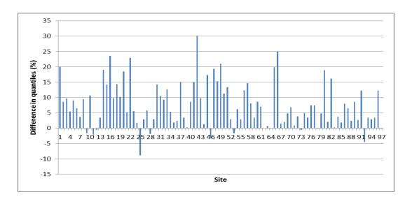
Figure 2.36 Differences in quantile estimates (expected quantiles from FLIKE) between CV = 0% and CV = 20% for 96 catchments in NSW (for 5% AEP flood)
