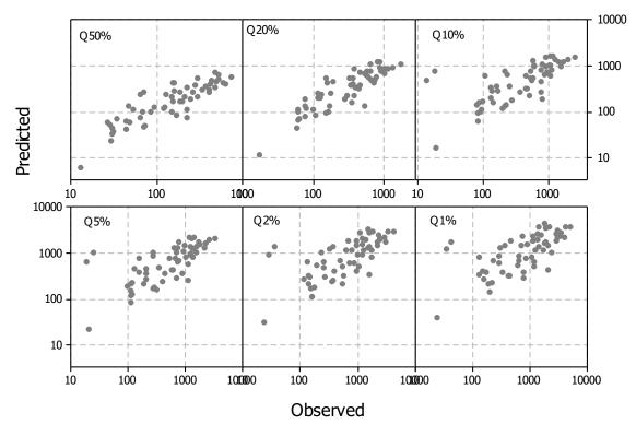
Figure B.6 Observed vs. predicted quantiles (in log space) for AEPs of 50% to 1% for Region 4 (NT + Kimberley WA) (flood discharges are in m³/s)
