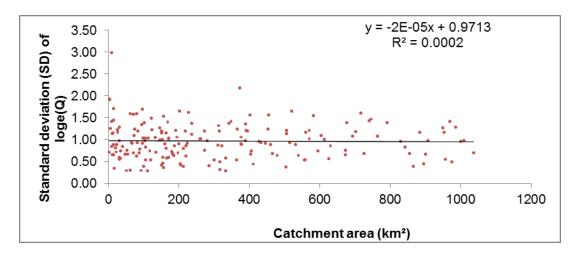
Figure 2.38 Relationship between SD of log<sub>e</sub>(Q) and catchment area for NSW 176 catchments
