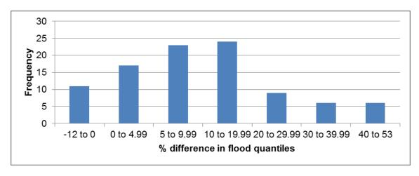
Figure 2.35 Difference in flood quantiles between CV of 0% and CV of 20% for 2% AEP flood quantiles (96 catchments from NSW)
