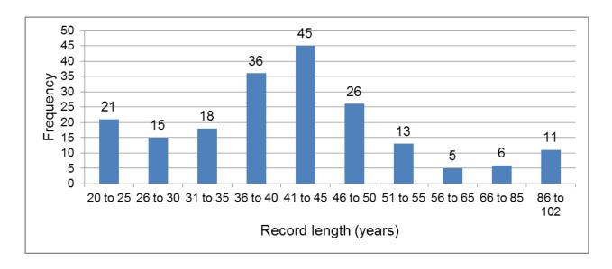
Figure 2.13 Distribution of streamflow record lengths of 196 stations from Queensland
