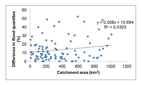
Figure 2.32 Catchment size vs. differences in flood quantile estimates between CV of 0% and CV of 20% for 96 NSW catchments (for 2% AEP flood)
