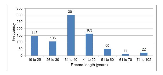
Figure 2.25 Distribution of streamflow record lengths of 798 stations from all data-rich areas of Australia
