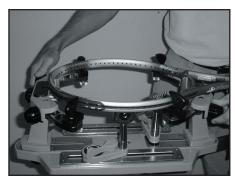
Turn the mounting arm adjustment knobs so that the angled frame support the fit up against the frame. The fit should be snug, but use caution. NOTE: Over-tightening can cause premature stress on the frame.
