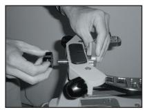
Loosen and remove the fine adjustment knobs, flip the head/throat frame supports so that they (supports) are each in an upward position. Replace the fine adjustment knobs.
