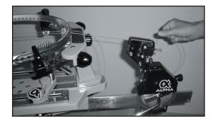
Take the 1st right main and load the string in the jaws of the gripper.
