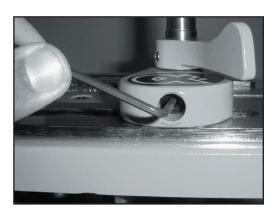
Turn the swivel base so that the outer port is aligned with the inner port. Take the 3mm allen key and insert into the internal adjustment screw. Turn clockwise to
