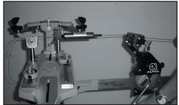
Clamp the fixed end of the tension calibrator. Load the string on the other end of the calibrator and pull tension. TIP: Make sure the clamp is positioned far enough from the tension head to allow a proper pull.
