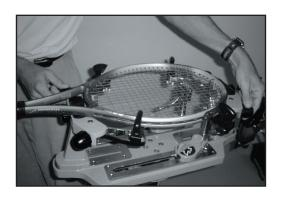
When the crosses are completed, tie off and trim the excess string. To release the racquet, release the pressure on the mounting knobs by loosening the adjustment knobs counter clockwise.
