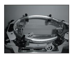
When stringing the mains, alternate by pulling one main on each side. Never pull two mains at one time.
