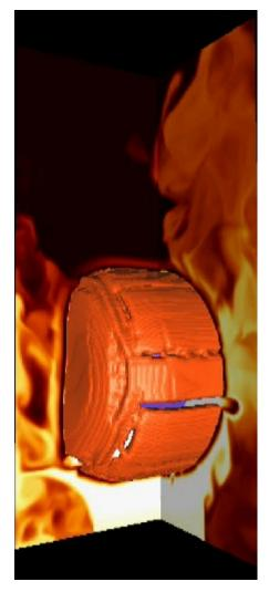
Figure 3: An example of and contemporary visualization simulation capabilities. Shown is a simulation of the explosion of a steel tank filled with explosive subjected to a jet of heated air. New methods are needed to capture multiscale effects and quantify uncertainties.
