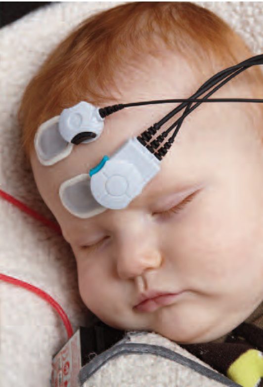
Figure 1. Amplitrode with built-in pre-filtering and amplification at the recording site.
