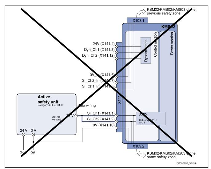
Fig. 7-9: Inadmissible single-channel wiring of IndraDrive Mi
