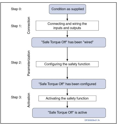
Fig. 8-4: Overview - commissioning steps of the "Safe Torque Off" function
