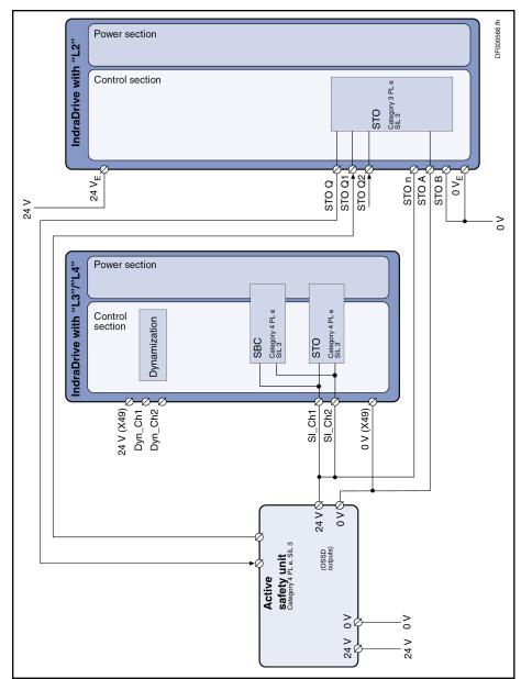
Fig. 7-19: Mixed Operation of Safety Options "L2" and "L3"/"L4" via an Active Safety Unit (Plus-Minus-Switching)
