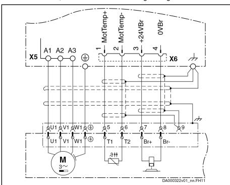
Fig. 12-1: Connection of motor temperature monitoring and motor holding brake
