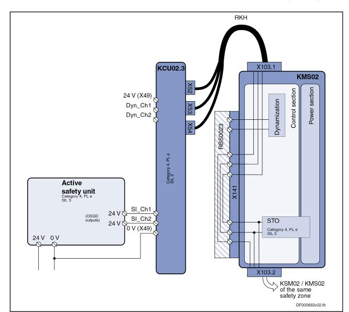
Fig. 7-11: KCU02 with active safety unit (plus-plus-switching outputs)
