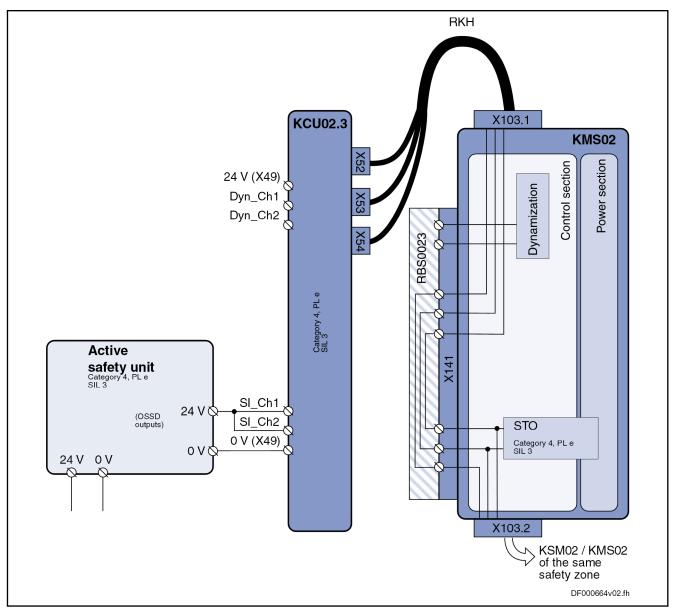
Fig. 7-12: KCU02 with active safety unit (plus-minus-switching outputs)
