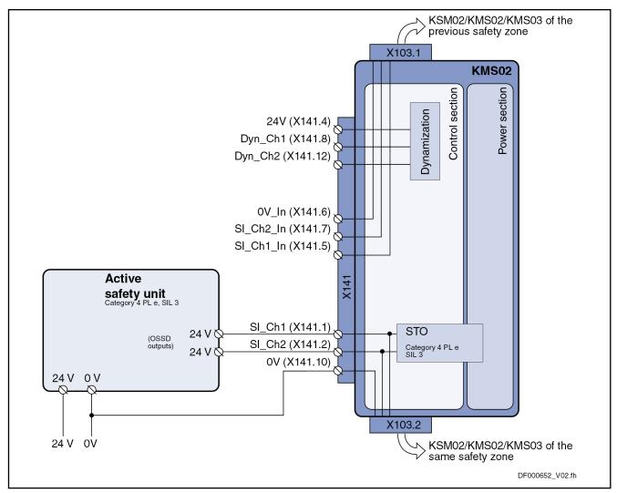
Fig. 7-16: KMS02 with active safety unit (plus-plus-switching outputs)
