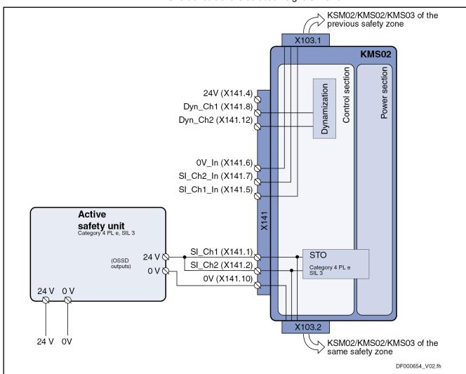
Fig. 7-15: KMS02 with active safety unit (plus-minus-switching outputs)
