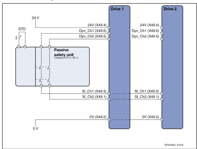
Fig. 7-7: Example of zone setup (in this case: 2 IndraDrive in a safety zone with dual-channel wiring and passive safety unit)
