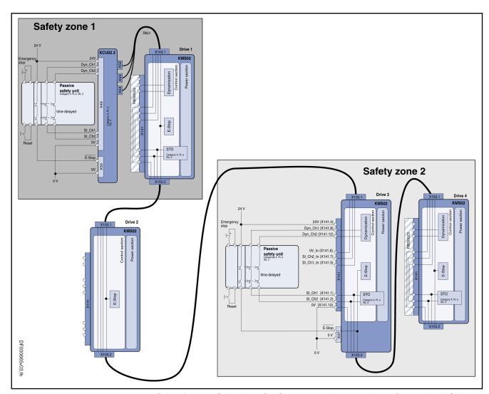
Drive 1 Selection of safety zone 1 via a passive safety unit at KCU;
