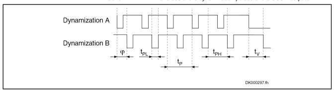
Fig. 5-2: Example of dynamized selection signals
