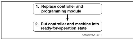
Fig. 9-2: Sequence of drive controller replacement
