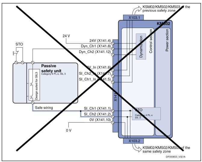
Fig. 7-8: Inadmissible single-channel wiring of IndraDrive Mi
