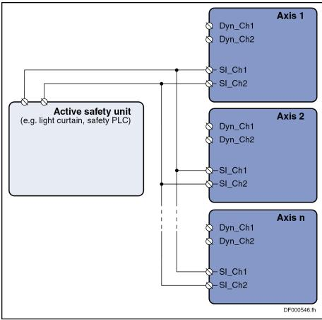
Fig. 5-3: Dynamization in the case of selection via an active safety unit
