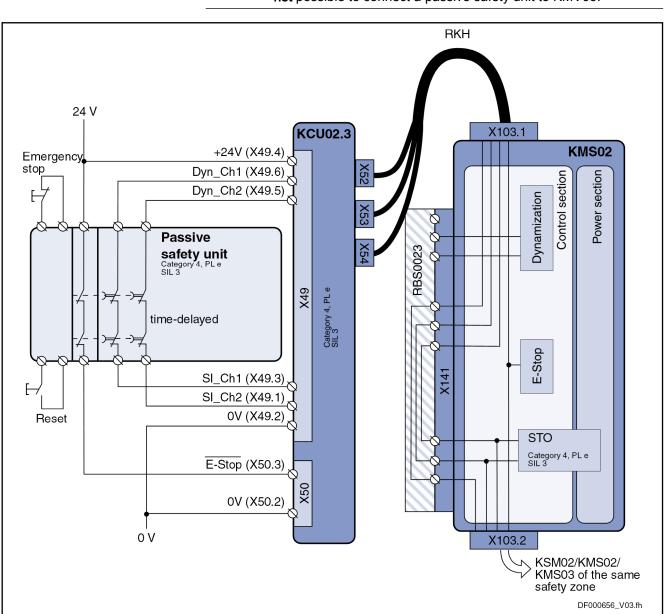
Fig. 7-13: SS1 function via KCU02 with **dual-channel** wiring and **passive** safety
