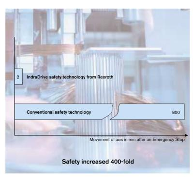
In the time it takes an operator in a protected area with conventional enabling to respond to an error, a linear axis with a ball screw spindle will have already covered a distance of 100 to 200 mm, and a linear motor a distance of 400 to 800 mm. IndraDrive safety technology detects the error within 2 ms and the axis moves a distance of no more than 2 mm.
