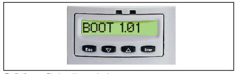
*Fig.7-42: Display with operating keys* The following figure shows the standard menu of the display:
