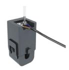
**2.** Place two-wire cable wires into clamps of current transformer. Fasten the clamps with cross-headed screwdriver.
