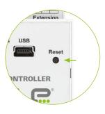
In case when change configuration of device is needed is necessary restart this device to factory settings using button Reset (press and hold 10 sec).
