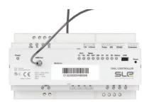
**3.** Connect the GSM and RF antenna plug to the Owl Controler and fasten it.
