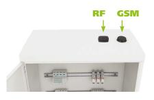
**2.** Insert the GSM and RF antenna and fasten it by tightening the nut with the wrench.
