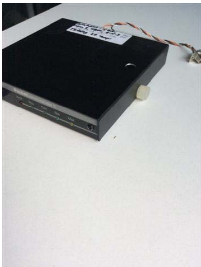
Speed screw on a TNC for rapid cabinet removal
