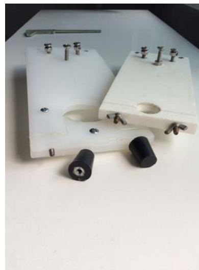
DIY Speed nuts enhance convenience to rapidly setup a large mobile antenna mount
