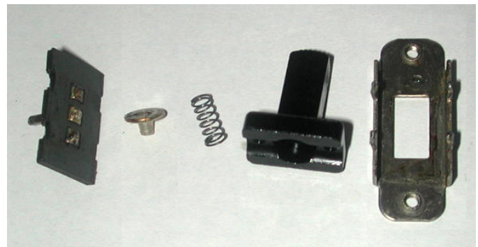
Figure 4: Disassembled Slide Switch parts. Left to right: Fiber plate with terminals and fixed contacts, disc contact, spring, plastic slider and metal switch frame.
