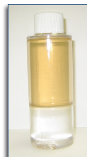
Fai Filtri's line of air compressor lubricants resist water contamination; typically separating in two distinct layers.
