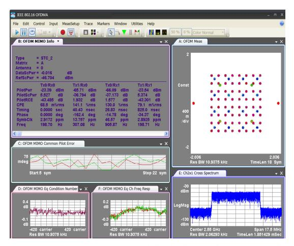
Save a signal and analyze it later with all the Option 89601BHTC tools. The cumulative history display format (Trace C), highlights signal performance over long periods. Place a marker on any point, particularly a transient outlying point, to determine its density of occurrence.
