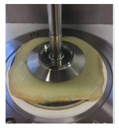
Figure 6. Raclette cheese after heating to 90°C followed by subsequent cooling to 20°C at a rate of 0.5°C/min. (Photo: Reidar B. Schüller)
