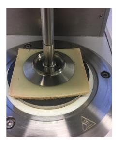
Figure 5. Raclette cheese placed on the Peltier plate before heating. The plate was lowered until the normal force was 10 mN. The gap was then locked in this position during heating to 90°C at a rate of 0.5 °C/min. (*Photo: Reidar B. Schüller*)
