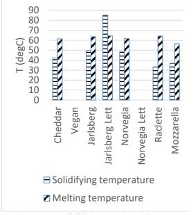
Figure 4. Solidifying- and melting temperatures for the different cheeses investigated (Vegan and Norvegia Lett remained viscoelastic solids at all temperatures. They did not melt at temperatures below 90°C).
