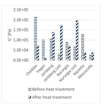
Figure 1. Elastic modulus in cheese at 20 °C before- and after heat treatme
