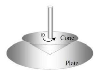
Figure 1 – A Cone & Plate measurement system
