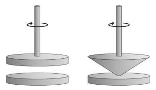
Figure 2 - Cone & Plate vs. Parallel Plate Measurement Systems
