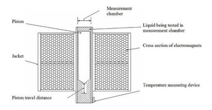
Figure 5 – A rendering of an Oscillating Piston Viscometer
