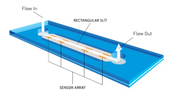
Figure 6 - Schematic of VROC® rectangular slit microfluidic cell
