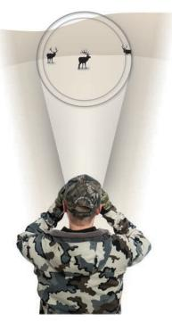
A wide field of view has advantages when following fast-moving action or scanning dense habitats. When comparing optics with the same size objective lenses, higher magnifications will generally have a narrower field of view.
