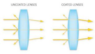
$\boxdot TIP$  The application of more coatings results in an increase of light transmission, resolution, contrast, and color fidelity.
