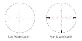
SFP - This style of reticle does not change size when magnification is changed. The advantage to this style of reticle is that it always maintains the same ideal visual appearance and will not appear "too fine" at low magnification or "too heavy" at high magnifications.
