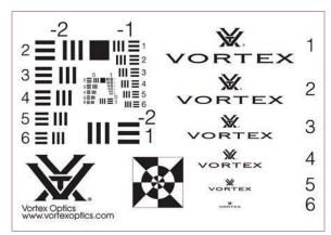
$\square$  **TIP** Use a resolution chart to determine how well a binocular, spotting scope, or riflescope can resolve fine details.
