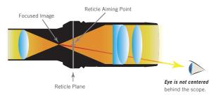
**»** When the target image is **not focused** on the reticle plane and your eye is **centered directly** behind the scope, no parallax occurs. This is because the line of sight from the eye to the focused target image **coincides** with the reticle aiming point.
