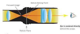
**Tip** Correctly focus the target image so it falls on the same optical plane as the reticle within the riflescope.
