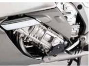
those essential characteristics. But surprisingly, the 160 hp six-cylinder 'drive-by-wire' engine is very pure in its design and, although it has four valves per cylinder, the cam timing is fixed and the cylinders are fed through a single throttle body with multipoint injection and long ram pipes. This helps to promote torque and flexibility. This is an ideal configuration for a touring bike, which must deliver fuss-free and accessible performance to the rider for hours on end.
