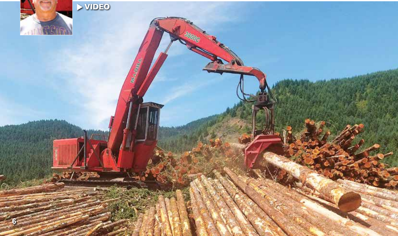
Operator Jesse Rice processes logs with a Madill 3800C equipped with a Waratah HTH624C processor. "The power gives me the ability to process a high volume of logs per day; it never slows down," said Jesse of the 3800C. "I can grab a log, cut the butt off, swing and feed at the same time. The new computerized Waratah head plays a big role in that too. It's fast and handles big wood with a feed rate of about 19 feet per second, so I can eat through a pile of timber quickly."
