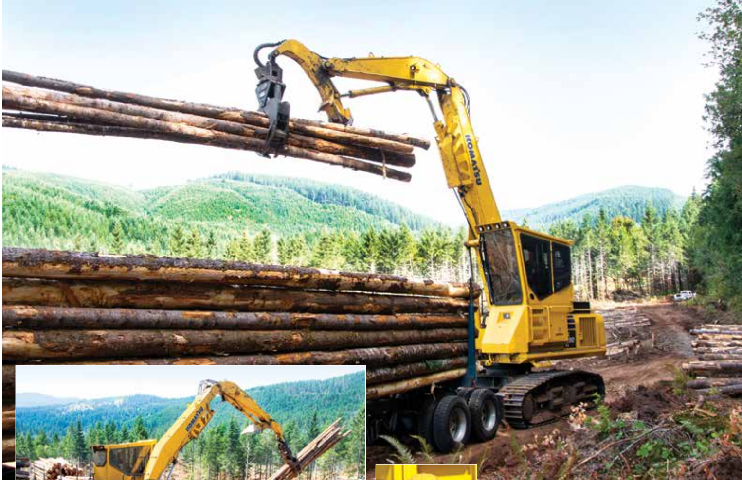
Operator Tom Lewison loads a truck and grabs another load of timber with a Komatsu PC290LL-11 equipped with a 58-inch grapple. "The hydraulics are very smooth, so it's comfortable to operate. The visibility is really good. There are no blind spots; so I can see the tracks, which makes it better for spotting things like stumps that you don't want to run over."
