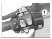
Press button 1 to switch on the hazard warning flashers.
