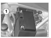
• Disconnect battery negative lead **1** and remove the battery.
