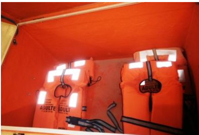
53- Life jackets and life vests should have the vessel name and reflectors. All life saving equipment should be listed and numbered for easy inspection.
