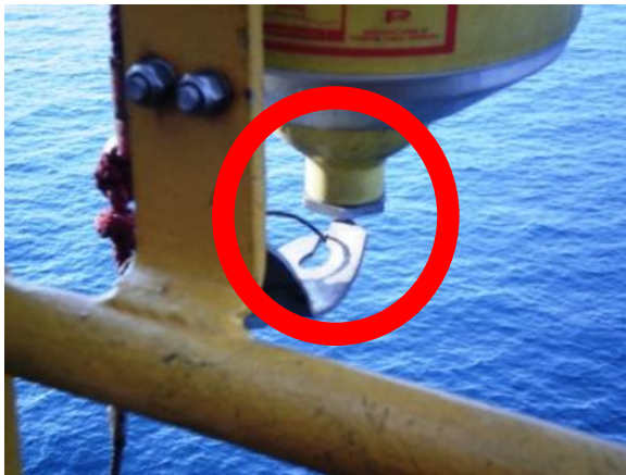
52- Bracket for the smoke buoy on port side is damaged and the pin to hold the ring buoy in the box is missing. A substitute pin should be installed to avoid losing the buoy.
