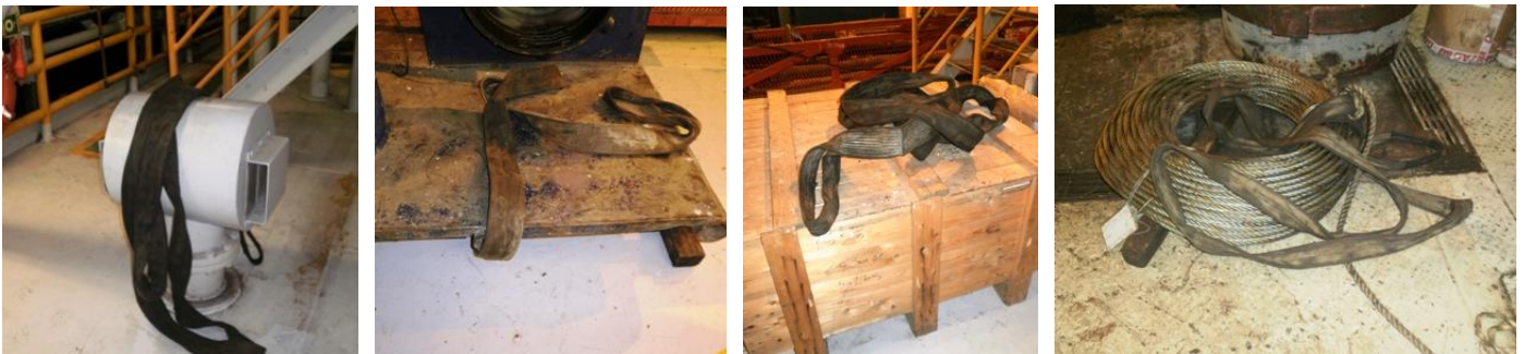
56- Un-controlled use of nylon straps should be avoided. Nylon straps should only be used under a PTW. Review Policy SAF 360.00 on synthetic web slings
