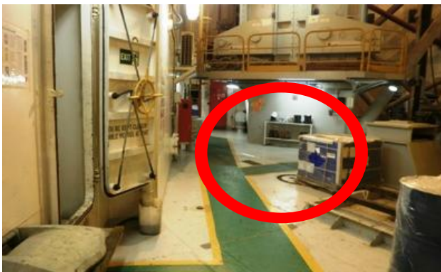
47- The hard hat and shoe racks are placed on the main deck a good 30 feet from the entrance to the accommodation. Areas outside the accommodation are PPE required areas and these racks should be moved inside the access doors to the accommodation so that crew can exit the accommodation with their PPE on. The current arrangement exposes crew to a hazard without PPE on deck.
