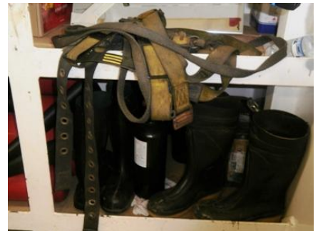
54- PPE and safety equipment like lanyards and safety belts should be kept in a designated areas and not stored with heavy equipment PPE boxes should be provided for crew to store their PPE in various areas of the rig.
