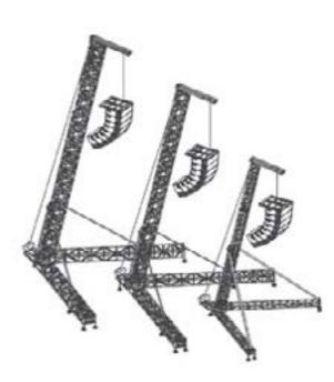
Total Structures designed V-Tower (sky-hook) as a single point lifting device. Main design is to lift audio Array speakers or any speaker cabinet or a number of other lifting uses, to a height of 30'. The sky-hook has 3 designed lifting points. Closest pick-point to the tower can lift 1,800lb., middle pick-point can lift 1,500lb., and the furthest pick-point out can lift 1,200 lb. wind loads up to 35 mph (with standard set-up).
