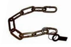
CM Special Theatrical Alloy Chain (STAC) is used for theatrical rigging applications where an adjustable bridle is required. Made from heat treated alloy steel to provide long life, each link is proof tested to assure weld and material integrity. The 4:1 design factor meets NACM/GR80 standards for strength. Pieces are tagged with grade, reach, size and working load limit for positive easy identification. The link accepts shackles up to 3/4". WLL12,000lbs.
