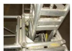
The medium duty truss sleeve block guides the attached medium duty truss as it is raised in a ground support system. Ground support system uses 12" x 12" towers. A sleeve block can also serve as a 4 way corner block.
