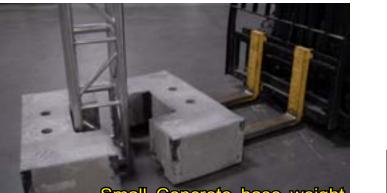
Small Concrete base weight per half, is 567 lb. (shown) Large Concrete base weight, per half, is 764 lb.
