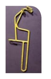
A simple, safe tool to replace the "snub knot" and be sure the arbor and pipe do not move while loading or unloading the counter weight. Like a "snub knot, this tool can be used to control movement with an imbalance. The maximum imbalance must not exceed 75lb.
