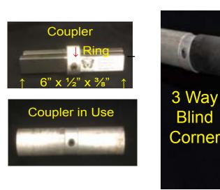
Quickly joins two pipes together without drilling or threading for permanent or temporary installations. The coupler is the same diameter as the pipe for a flush appearance. IHP can provide additional ring sizes to match your needs. Install by loosening the set screw with a ¼" hex key to open the splice. Insert the coupler completely into both pipes and tighten the set screw.
