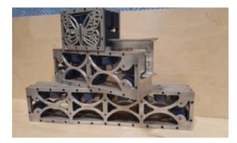
Top trolley is 12" long Middle trolley is 24" long Bottom Trolley is 36" long All made to fit 3" x 6" aluminum I-Beam
