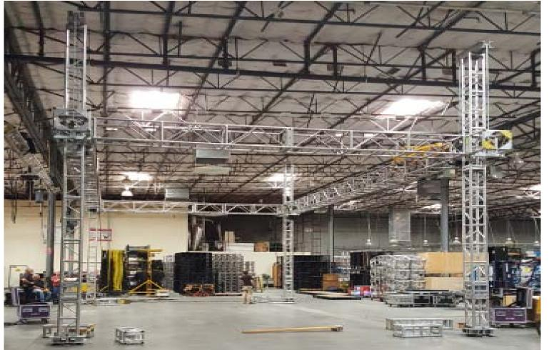
This is an example of a ground support system which can be used inside or outside. This
