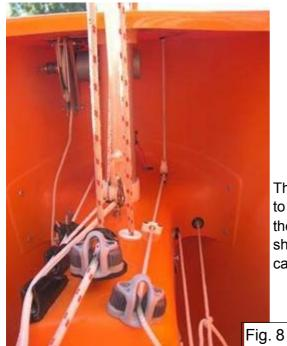
The jib sheet is 2 part which gives the option of one end going to a servo assist winch and the other down to the camcleat on the starboard side of the console for manual operation. (fig 8 shows the jib sheet winch behind mast, jib sheet and camcleat).
