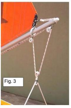
A boom vang is fitted which prevents the boom skying when running in fresh to strong winds. (see fig 4)
