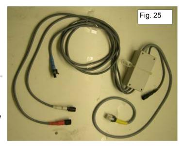
2 leads running aft, (1) the larger of the 2 passing through the aft bulkhead, via a 32mm single hole rubber bung, its yellow 9 pin plug connecting to the joy- stick. (2) The smaller of the 2 aft leads plugs into the helm winch lead (black plugs) which should always be hanging on a hook just aft of the starboard side inspection port.
