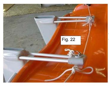
Remove the spring clips and pass the clevis pins up through the holes at the end of the tillers. Re-insert the spring clips. (fig 22)
