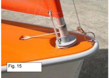
At the bow is the jib strut downhaul, free it and attach its plastic hook to the lug on the front of the claw. (fig 13—page 14).
