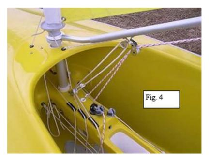
The mainsail outhaul primarily cleats at the boom, (fig 5) but passes thru a deckeye just behind the main mast, down to the console and turns through the boom vang/ outhaul double becket block and back to the central of the 3 clamcleats on the port side of the console. (fig 6)
