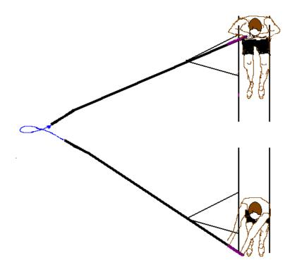
This blade does not slip much in the direction perpendicular to the shaft. Outboard length must be decreased to achieve optimal load. (i.e. force, speed, and angles at catch and finish)
