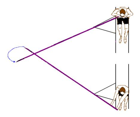
This blade slips a lot in the direction perpendicular to the shaft. The outboard must be longer to achieve optimal load. (i.e.optimal force, speed, and angles at the catch and finish)
