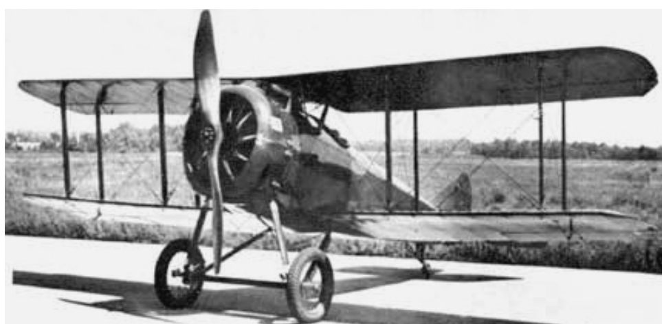
The last American aircraft produced before the end of the First World War, the Standard E-1 entered service in early 1918 but never saw combat. Although it was stable and maneuverable, it proved too slow and underpowered for use as a fighter. Instead, the United States Air Service accepted it for use as an advanced trainer.
