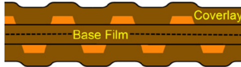
Figure 4.8 Staggered adjacent-layer traces are preferred
