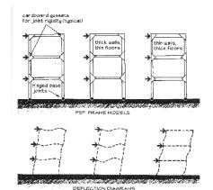
Figure 9.19: Model demonstration of the effects of varying the stiffness of beams and columns when a building frame is subjected to lateral loads.
