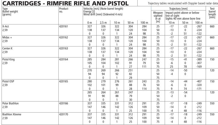
Ballistic coefficients are calculated by Quick Target Unlimited Lapua Edition from  $V_0$  to  $V_{75}$  BC G1 for all Rimfire .22 LR bullets = 0.172
