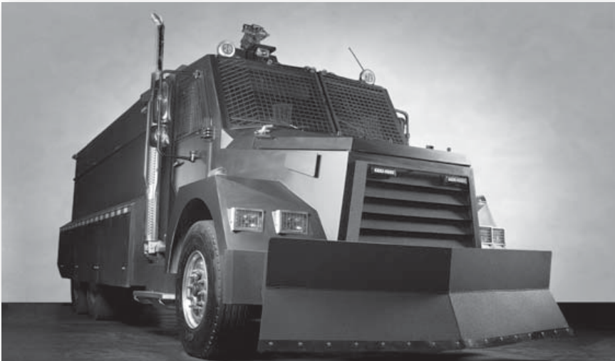
Another view of the INKAS Armored Riot Control Vehicle. Wire-mesh protection is provided on all windows, and the bodywork has ballistic protection up to 7.62x54mm/.308 Winchester. Door and window apertures are overlapped to avoid presenting crowbar-friendly attack points. (INKAS)
