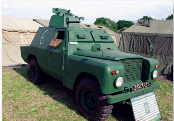
The Mk 1 Shorland armoured car. This is the original 'boat tail' Shorland, which had a crew capacity of just three people. Later versions extended the personnel capacity to eight people (two crew up-front plus six in the rear). (Geni)
