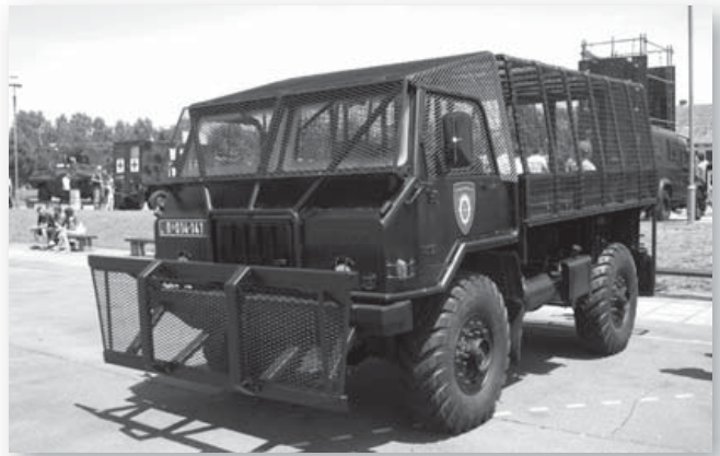
The TAM 110 is a light RCV used by the Serbian Gendarmerie for riot control. The rear cage acts as both a protective shield for officers and an improvised holding cell for apprehended rioters. (Boris Dimitrov)
