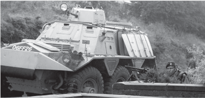
An Alvis Saracen sits outside a house in Londonderry in 1972, waiting for trouble. This is a turreted version, fitted with a 7.62mm machine gun. Note the extensive barricade ram at the front and the wire mesh covering the headlamps. (Press Association)
