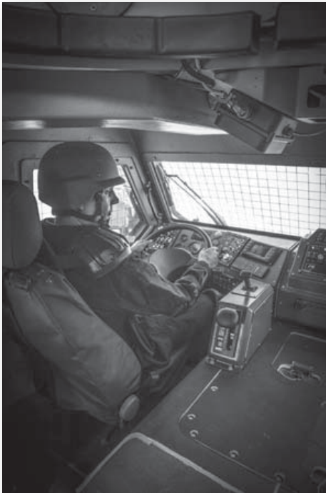
The driver's position in the Paramount Group Maverick. The driver can centrally control the tyre pressure, lower/raise the pneumatic dozer blade and bullbars and also monitor the rear of the vehicle via cameras linked to internal monitors. (Paramount Group)
