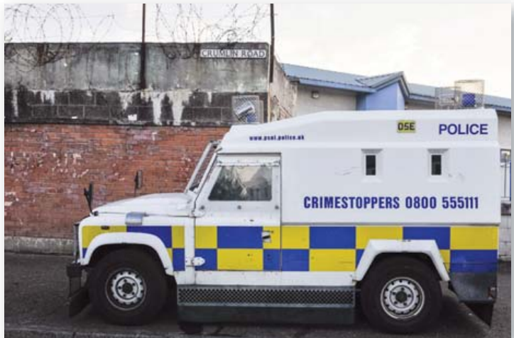
A Police Service of Northern Ireland (PSNI) Land Rover Tangi, 2013. Based on the Land Rover Defender 110 chassis, it is heavily armoured to protect from fire bombs and minor explosive devices. It is known as the 'meat wagon' in Northern Ireland. (Press Association)
