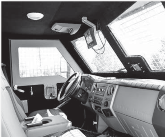
The forward cab of the Paramount Maverick. Note how the windows are covered with wire mesh. Although the windows themselves are bulletproof, the mesh protects them further from thrown and hand-held weapon impacts, and helps to maintain occupant visibility. (Paramount Group)
