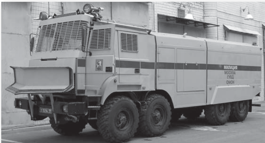
The Lavina-Uragan (Avalanche-Hurricane) is used by the Moscow OMON security forces, plus other law enforcement agencies in Russia and the former Soviet Union. It is based around a Ural-532362 chassis. (Vitaly Kuzmin)
