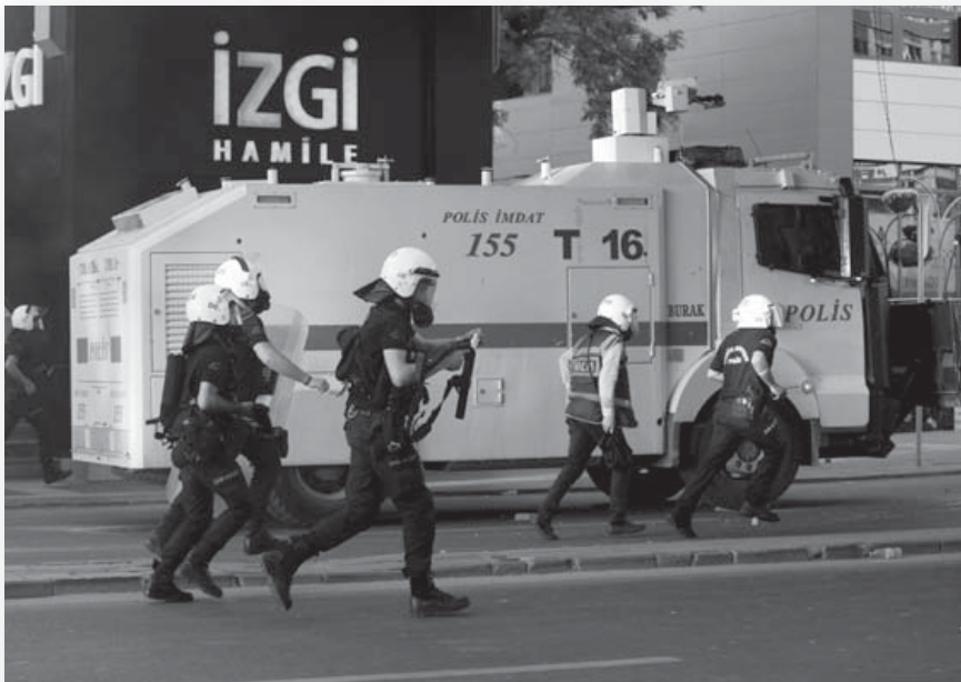
A Turkish water-cannon vehicle, manufactured by Katmerciler Arac Ustu Ekipman Sanayi & Ticaret AS (KATMR), here seen combatting demonstrations in Ankara in May 2014. It has a single top-mounted water jet, capable of firing pulses or solid jets. (Press Association)
