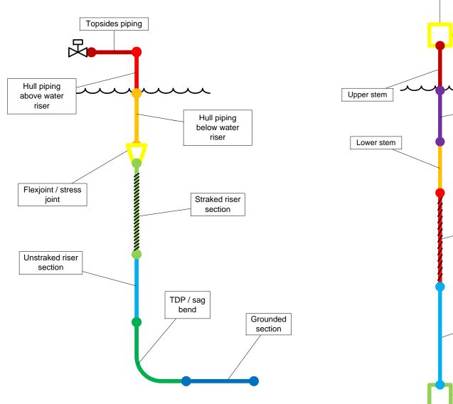
Surface Flexible production/ gas lift/ injection tree jumper Buoyancy can Straked riser section Unstraked riser section Subsea wellhead, 6of 21 conductor
