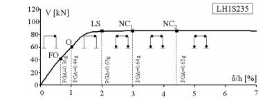
Figure 3 Example of pushover curve for the determination of the earthquake-induced damage
