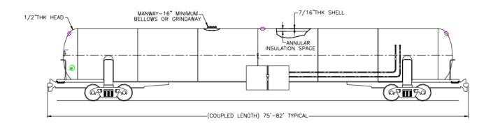
Cutaway Drawing of Tank Car (Courtesy of Chart Industries)
