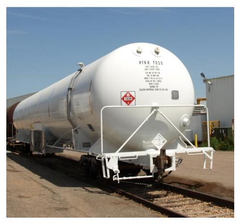
Figure F.6 DOT 113 Rail Tank Car (Back End)
