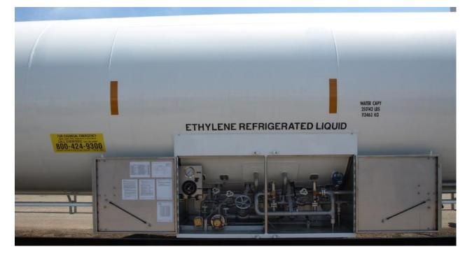
Figure F.7 DOT 113 Ethylene Tank Car Valve Details
