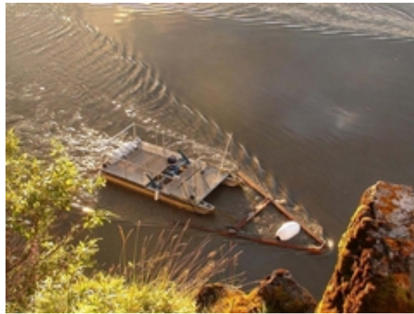
Figure 11: Debris boom on 5 kW Encurrent Turbine in Ruby, Alaska (Yukon River Inter-Tribal Watershed Council , 2008)
