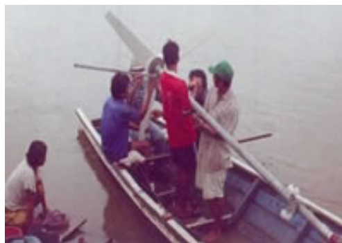
Figure 10: Furling of micro-hydrokinetic battery-charging device (Hands On: The Earth Report, 2004)
