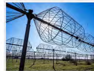
Cage dipole antennas in the Ukrainian UTR-2 radio telescope. The 8 m by 1.8 m diameter galvanized steel wire dipoles have a bandwidth of 8–33 MHz.
