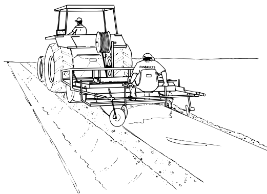
Figure 4.7 Simultaneous Installation of Drip Tape and Plastic Mulch
