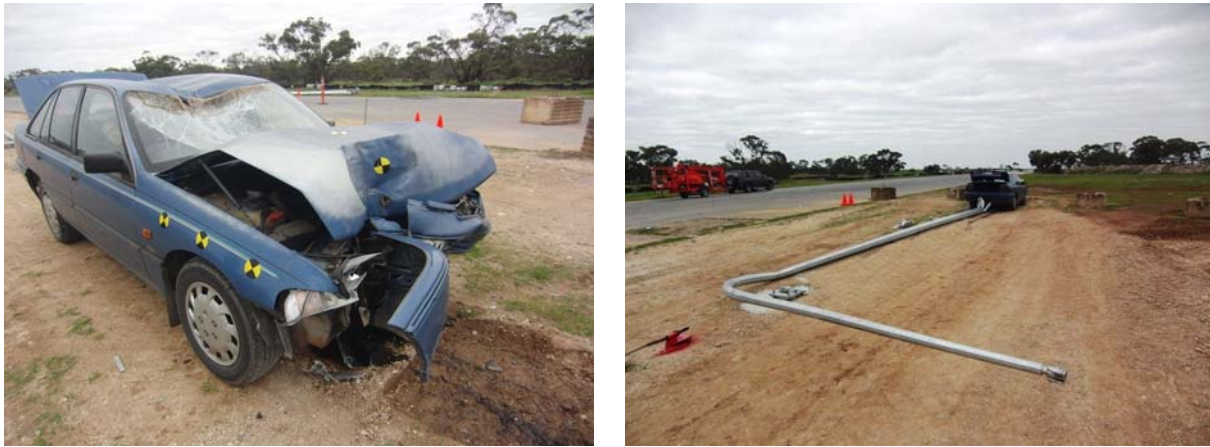
FIGURE 10 Impact test of 1,500-kg vehicle at 70 km/h.
