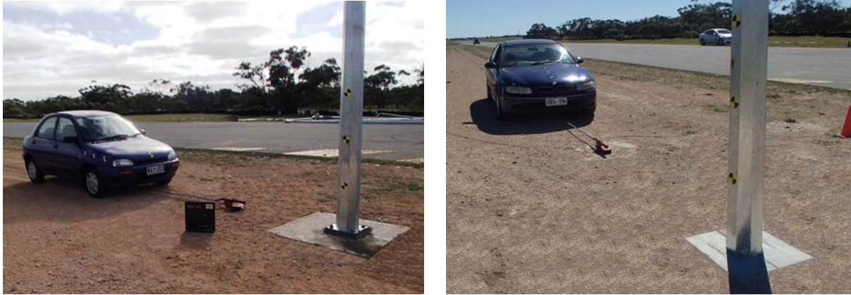
FIGURE 7 Test with lowered base plate.
