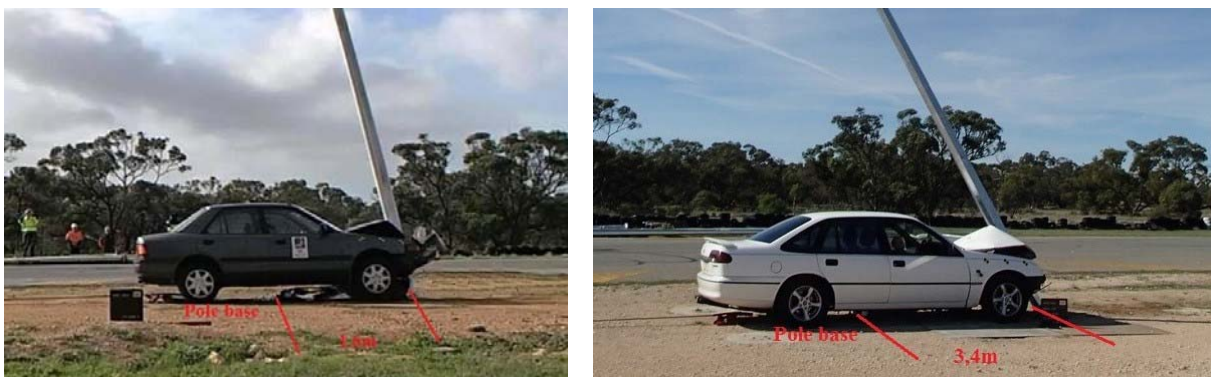
FIGURE 11 Impact test of 1,500-kg vehicle at 70 km/h.
