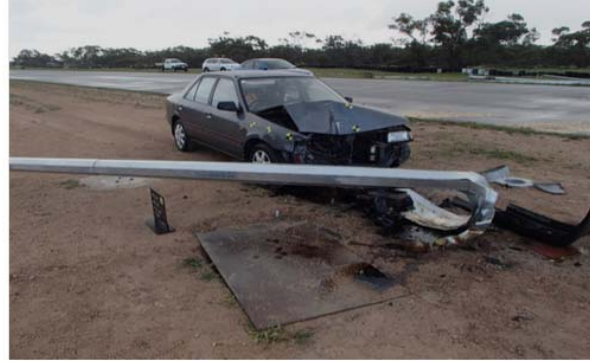
FIGURE 1 The pole should collapse in a predictable manner.
