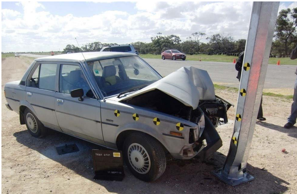
FIGURE 9 Impact test of 1,100-kg vehicle at 50 km/h.
