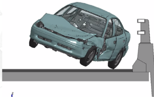
FIGURE 11 Finite element calculation for the Australian VRS-MAO system.
