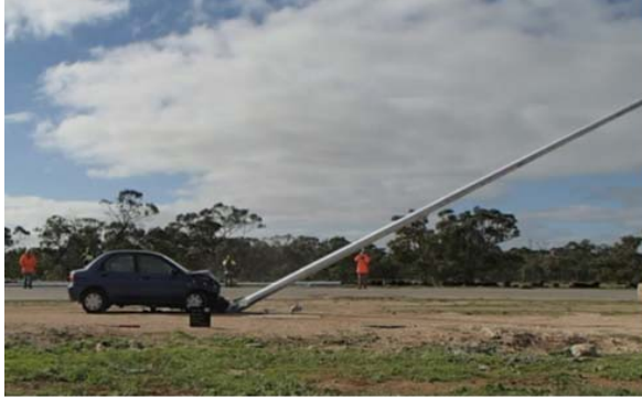
FIGURE 1 The pole should collapse in a predictable manner.
