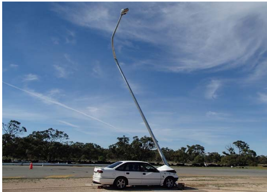
FIGURE 6 Test with strengthened attachment of the luminaire.
