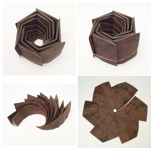
Fig. 21 A wood veneer laminate fabricated constant-height flasher for m = 6 , n_r = 9 , \varepsilon = 3 deg, and h = 4.8 . Top left: stowed state, top view. Top right: stowed state, side view. Bottom left: partially folded. Bottom right: deployed.
