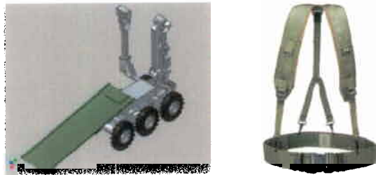
Figure 4: Left: Conceptual drawing of REX with deployed stretcher. Right: Load Bearing Equipment harness for patient extraction.
