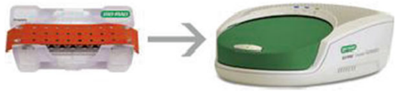
Fig. 6 The droplet generator cartridge covered with gasket inserted into the droplet generator. The processing of eight samples takes about 2 min. Post-processing, the droplets are transferred to a 96-well plate
