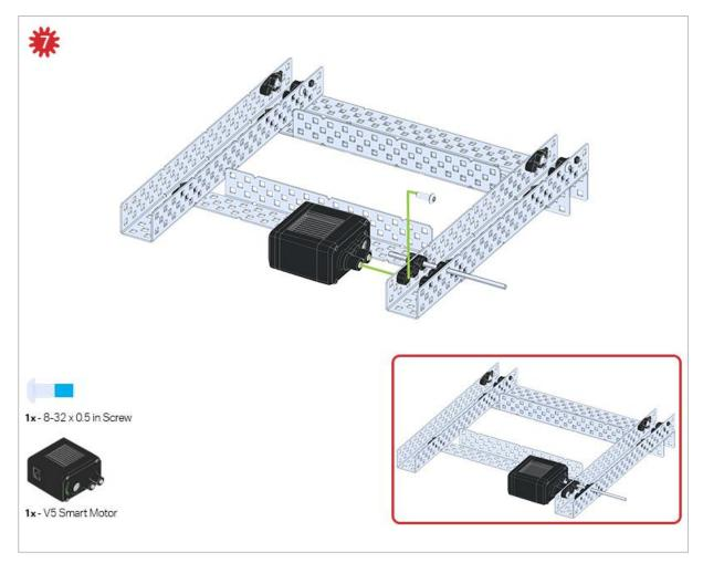
Make sure your Smart Motors are oriented in the correct direction (screw holes facing the outside of the build and the shaft hole towards the inside).
