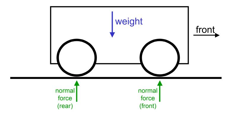
The <u>normal force</u> is the force that the wheels exert on the floor, and is equal and opposite to the force the floor exerts on the wheels. In the simplest case, this is dependent on the <u>weight</u> of the robot. The normal force is divided among the robot features in contact with the ground.
