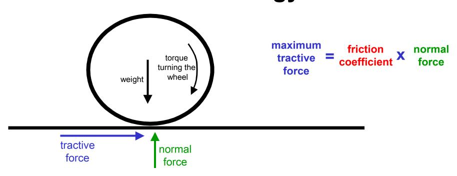
The <u>friction coefficient</u> for any given contact with the floor, multiplied by the <u>normal force</u>, equals the maximum <u>tractive force</u> can be applied at the contact area.
