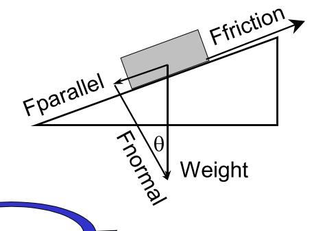
When  $F_{friction} = F_{parallel}$ , no slip
