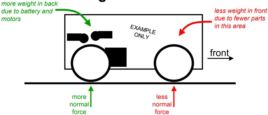
The weight of the robot is **not** equally distributed among all the contacts with the floor. Weight distribution is dependent on where the parts are in the robot. This affects the normal force at each wheel.
