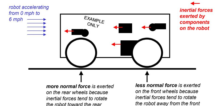
In an extreme case (with rear wheel drive), you pull a wheelie In a really extreme case (with rear wheel drive), you tip over!
